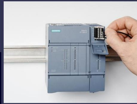
Removable high(er) density terminal blocks with push-in wiring for ease of use → non-contact pre-wiring position.
